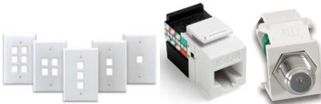
The 8-pin modular jacks (RJ-45) must use the TIA/EIA 568 A pin out standard (most outlets have both color codes printed on them 568 A and B) in order to meet industry certification and cabling standards. Combination 8-pin modular & F-connector jacks (e.g. Leviton / Belden/CDT MDVO multimedia module) may be installed at each location.
