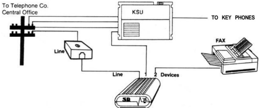
You can only install your SR on the CO\* side of the KSU. You cannot install it on the station or extension side.
