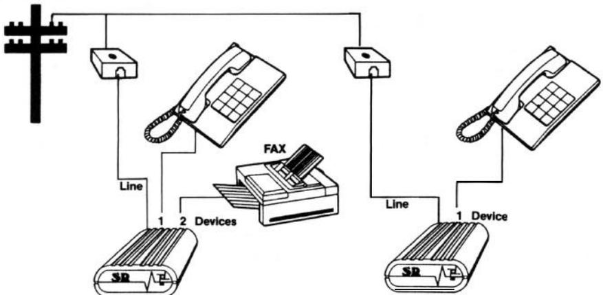
If total ring supervision is required for more than one phone, and barge-in protection is not needed, buying additional SR Call Processors may be less expensive than changing your wiring, especially if your site is wired in a user-unfriendly way, or if your extensions are in other buildings.
